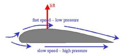
The air splits over the front of the wing known as the leading edge. As the air moves under the wing nothing happens to it but as it moves over the top of the wing the air is accelerated and moves faster. This causes a decrease in air pressure on top of the wing, and because there is now a higher pressure underneath the wing it pushes upwards and creates lift.
