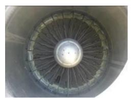
A major source of Foreign Object Damage is from **bird strikes**. At high speed, the impact of a bird hitting an aircraft may crack a window, or damage an engine, causing it to fail. Many airfields take special measures to reduce the risk of bird strikes, such as using loud noises to scare birds away. Airfields located close to large bodies of water, to
