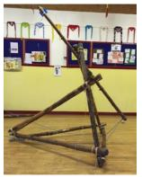
**Step 4:** Place your ammunition (tennis or sponge ball) in the plastic cup and fire the catapult by pulling sharply on the two lengths of rope. You may find that altering the angle at which you pull the ropes changes the distance your ammunition will travel.
