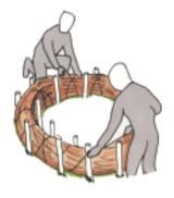
First place a number of stakes in the ground and then pile light twigs and branches between the stakes, to make a doughnut shape. When the shape is complete weave sisal or rope around the pile to keep it together.
