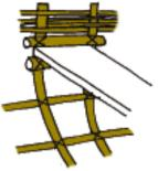
The seat is fixed in the middle of the coracle. Bind the edge of the seat to the frame.
