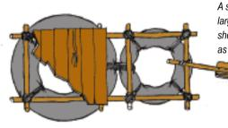
A similar raft can be made with a large and a small inner tube as shown. Either make a baseboard as above or construct a frame to hold the inner tubes together.
